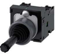
Coordinate switch, 22 mm, round, plastic with metal front ring, black, 2 switch positions, vertical, momentary contact type, with mechanical interlocking in O position, with holder, 1 NO, 1 NO, screw terminal, with laser labeling, inscription or symbol Customer-specific selection with SIRIUS ACT configurator (CIN)
