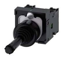
Coordinate switch, 22 mm, round, plastic, black, 2 switch positions, vertical, momentary contact type, with mechanical interlocking in O position, with holder, 1 NO, 1 NO, screw terminal, with laser labeling, upper case and lower case, always upper case at the beginning of the word
