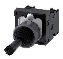
Coordinate switch, 22 mm, round, plastic with metal front ring, black, 2 switch positions, vertical latching, without mechanical interlocking, in O position, with holder, 1 NO, 1 NO, screw terminal, with laser labeling, lower case
