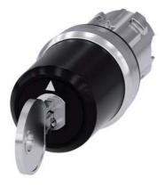
key-operated switch Siemens, 22 mm, round, metal, shiny, lock number SSG10, with 2 keys, 3 switch positions I-O<II, left latching, momentary contact type on the right, actuating angle 2x45°, 10:30h/12h/13:30h, key removal I, with laser labeling, lower case
