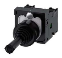
Coordinate switch, 22 mm, round, plastic, black, 2 switch positions, horizontal latching, without mechanical interlocking, in O position, with holder, 1 NO, 1 NO, screw terminal, with laser labeling, inscription or symbol, Customer-specific selection with SIRIUS ACT configurator (CIN)
