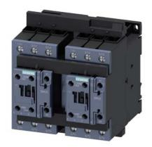
Reversing contactor assembly AC-3, 22 kW/400 V, AC/DC 20-33V 3-pole, Size S2 screw terminal electrical and mechanical Interlock 2 NO integrated
