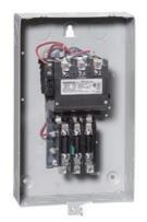
Non-reversing motor starter, Size 2 1/2, Three phase full voltage, Amb compensate bimetal OLrelay Contactor amp rating 60Amp 110 120/220 240VAC 60HZ coil, Non-combination type, Enclosure type 1, Indoor general purpose use
