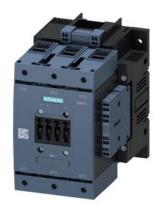
Power contactor, AC-3 115 A, 55 kW / 400 V AC (50-60 Hz) / DC operation 23-26 V UC Auxiliary contacts 2 NO + 2 NC 3-pole, Size S6 with box terminals Drive: conventional Spring-type terminal
