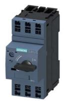
Circuit breaker size S00 for motor protection, CLASS 10 A-release 2.8...4 A N release 52 A Spring-type terminal Standard switching capacity
