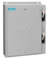
Duplex starter W/O alternator Size 1 Three phase full voltage Solid-state overload relay OLRelay amp range 10-40a 110VAC 50HZ / 120VAC 60HZ coil Combination type Two 30A circuit breakers Encl NEMA type 4X 304 S-steel Water/dust tight non-corrosive
