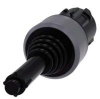
Coordinate switch, 22 mm, round, plastic with metal front ring, black, 2 switch positions, vertical latching, with mechanical interlocking, with laser labeling, upper case
