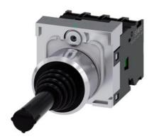
Coordinate switch, 22 mm, round, metal shiny, black, 4 switch positions, momentary contact type, without mechanical interlocking, in O position, with holder, 1 NO, 1 NO, 1 NO, 1 NO, screw terminal, Z=20-unit packaging
