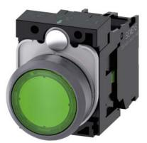
Illuminated pushbutton, 22 mm, round, plastic with metal front ring, green, pushbutton, flat, momentary contact type, with holder, 1NO, LED module with integrated LED 24 V AC/DC, screw terminal, with laser labeling, symbol number according to, ISO 7000 or IEC 60417
