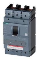
CIRCUIT BREAKER 3VA5 UL FRAME 400 BREAKING CAPACITY CLASS C 100kA @ 480 V 3POLE, LINE PROTECTION TM230, FTAM, In=250A OVERLOAD PROTECTION IR=250A FIXED SHORT CIRCUIT PROTECTION II=5...10 X IN UL489 SB (NAVAL), 50 DEG CEL. W/O CONNECTION
