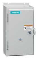
Non-reversing motor starter, Size 2 1/2, Three phase full voltage, Solid-state overload relay, OLRelay amp range 25-100A, 24VAC 50-60HZ coil, Non-combination type, Enclosure type 12, Dust/drip proof for indoors, Standard width enclosure
