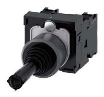
Coordinate switch, 22 mm, round, plastic with metal front ring, black, 2 switch positions, horizontal, momentary contact type, without mechanical interlocking in O position, with holder, 1 NO, 1 NO, screw terminal, Z=20-unit packaging
