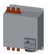
SIRIUS soft starter Values at 460 V, 50 °C standard: 551 A, 450 hp Inside-delta: 954 A, 850 hp 200-460 V AC, 115 V AC spring-type terminals !!! Phased-out product !!! Successor is SIRIUS 3RW5, Preferred successor type is >>3RW5552-2HA14<<
