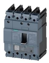
circuit breaker 3VA5 UL frame 125 breaking capacity class H 65kA @ 480V 4-pole, line protection TM230, FTAM, In=50A overload protection Ir=50A fixed short-circuit protection Ii=5...10 x In N conductor unprotected without connection
