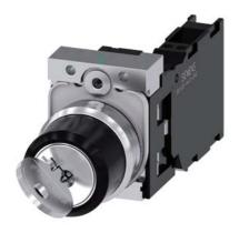
RONIS key-operated switches, 22 mm, round, metal, shiny, lock number SB30, with 2 keys, 2 switch positions O-I, latching, 90° operating angle, 10:30/1:30 o'clock, key removal O+I, with holder, 1NO+1NC, spring-type terminals, possible special locks: SB31, 421, 455, Z=20-unit packaging
