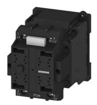
Contactor, Size 2, 2-pole, DC-3 and 5, 32 A Auxiliary contacts 22 (2 NO + 2 NC) 110V AC 50Hz/132V AC 60Hz AC operation
