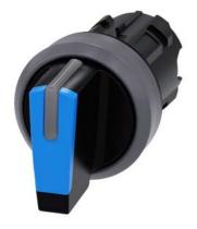
Selector switch, illuminable, 22 mm, round, plastic with metal front ring, blue, selector switch, short, 3 switch positions I-O<II, left latching, right momentary contact type, actuating angle 2x45°, 10:30h/12h/13:30h, with laser labeling, upper case and lower case, always upper case at the beginning of the word
