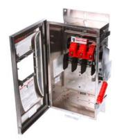
Siemens Low Voltage Circuit Protection Heavy Duty Safety Switches -Type ENCLOSED / SAFETY SWITCH Meets stds: UL. Built material: 316SSsingle throw action. Rated 600V (60A) at 60Hz.3-Pole. Insulated. TYPE 4X enclosure with 2 or 3 point mounting. No special features listed.
