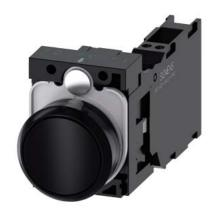
Pushbutton, 22 mm, round, plastic, black, pushbutton, flat, momentary contact type, with holder 1 NO+1 NC, spring-type terminal, with laser labeling, lower case
