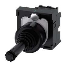
Coordinate switch, 22 mm, round, plastic, black, 2 switch positions, vertical latching, with mechanical interlocking, in O position, with holder, 1 NO, 1 NO, screw terminal,
