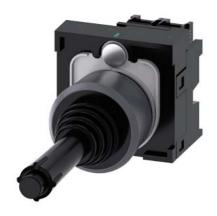
Coordinate switch, 22 mm, round, plastic with metal front ring, black, 2 switch positions, vertical latching, with mechanical interlocking, in O position, with holder, 1 NO, 1 NO, screw terminal, Z=20-unit packaging
