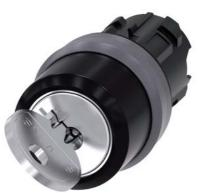
RONIS key-operated switch, 22 mm, round, plastic with metal front ring, lock number 455, with 2 keys, 2 switch positions O<I, momentary contact type, Actuating angle 45°, 10:30h/12h, key removal O, with laser labeling, upper case and lower case, always upper case at the beginning of the word
