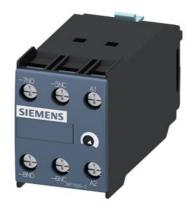
solid-state time-delayed front-side auxiliary switch Time range 5...100 s, 100 ... 127 V AC / DC, 1 NO contact, 1 NC contact OFF delay, without control signal for  $3\mathsf{RT1}$
