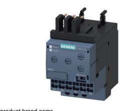
Monitoring relay, can be mounted to Contactor 3RT2, Size S00 basic, analog adjustment Apparent current monitoring 1.6-16 A, 20-400 Hz, 2-phase Supply 24 V AC/DC 1 change-over contact Monitoring for Current overshoot and undershoot Phase failure, Cable break with or without fault buffer ON delay 0-60 s Noise pulse suppression 0-30 s Switching hysteresis 6% spring-type connection system
