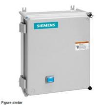
Non-reversing motor starter, Size 2 1/2, Three phase full voltage, Amb compensate bimetal OLrelay Contactor amp rating 60Amp 110 120/220 240VAC 60HZ coil, Non-combination type, Enclosure type 4X Fiberglass, Water/dust tight noncorrosive
