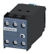
solid-state time-delayed front-side auxiliary switch Time range 0.5...10 s, 24 V AC/DC, 1 NO contact, 1 NC contact OFF delay, without control signal for 3RT1
