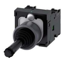
Coordinate switch, 22 mm, round, plastic with metal front ring, black, 2 switch positions, vertical, momentary contact type, with mechanical interlocking in O position, with holder, 1 NO, 1 NO, screw terminal, with laser labeling, upper case
