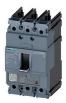
circuit breaker 3VA5 UL frame 125 breaking capacity class H 65kA @ 480V 3-pole, line protection TM230, FTAM, In=40A overload protection Ir=40A fixed short-circuit protection Ii=5...10 x In UL 489 SB (naval), 50° C without connection
