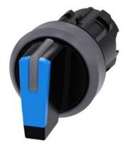
Selector switch, illuminable, 22 mm, round, plastic with metal front ring, blue, selector switch, short, 3 switch positions I-O<II, left latching, right momentary contact type, actuating angle 2x45°, 10:30h/12h/13:30h, Z=50-unit packaging
