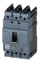
circuit breaker 3VA5 UL frame 125 breaking capacity class S 25kA @ 480V 3-pole, line protection TM230, FTAM, In=60A overload protection Ir=60A fixed short-circuit protection Ii=5...10 x In UL 489 SB (naval), 50° C without connection
