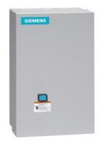
Non-reversing motor starter Size 2 1/2 Three phase full voltage Amb compensate bimetal OLrelay Contactor amp rating 60Amp 110VAC 50HZ / 120VAC 60HZ coil Non-combination type Enclosure NEMA type 1 Indoor general purpose use Extra-wide enclosure
