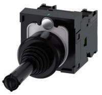
Coordinate switch, 22 mm, round, plastic, black, 2 switch positions, horizontal, momentary contact type, without mechanical interlocking in O position, with holder, 1 NO, 1 NO, screw terminal, with laser labeling, inscription or symbol Customer-specific selection with SIRIUS ACT configurator (CIN)
