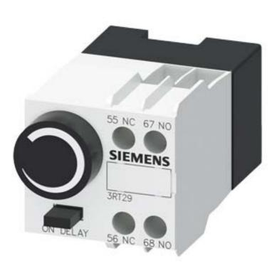
Note! Changed technical specification! See data sheet/declaration of compliance with the order Pneumatic timing relay block ON delay 1 ... 60 s 1 NO + 1 NC, for motor contactors size S0 according to DIN VDE 0116 !!! Phased-out product !!!
