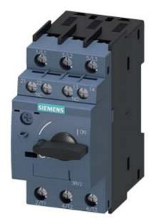
Special type Circuit breaker size S00 for motor protection, CLASS 10 A-release 3.5...5 A N release 65 A screw terminal Standard switching capacity with transverse auxiliary switches 1 NO+1 NC Ambient temperature -50 °C 500 switching cycles
