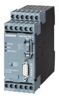
SIPLUS SIMOCODE pro V Basic unit 2 -25...+60°C with conformal coating based on 3UF7010-1AU00-0 . E- type with "Safety ""12 Mbit/s, RS485;""" "4I/3O freely parameterizable;" "US: 110-240V AC/DC; input for" "thermistor connection;" "monostable relay outputs;" expandable by extension modules
