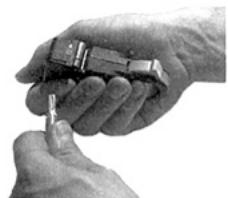
7. The removed insulation remains in the stripper. After releasing the clamp, the remnants can be removed.
