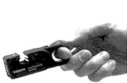
1. How to hold the insulation stripper in your **right hand**.
