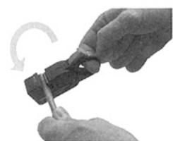
5. Rotate the stripper around the cable approx. 4 times for PVC-Insulation and approx. 8 times for PUR-, or PE-Insulation in the direction of the arrow.
