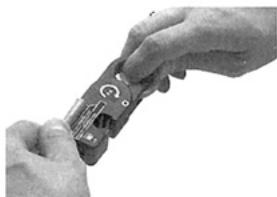
2. Match up the cable end with the template so that your left index finger is against the end surface of the tool.
