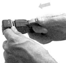
4. Clamp the cable **firmly** in the stripper.
