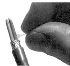
10. Pull the protective foil off the cores
