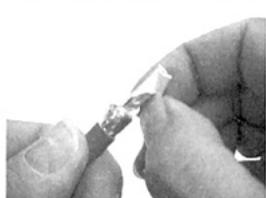
8. If the white filler does not come away with the insulation, remove it by hand.
