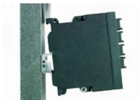
Figure 4-2 IE Switch X-200 removing from a DIN rail (35 mm)
