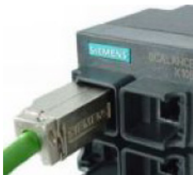
Figure 5-3 Inserting the IE FC RJ-45 Plug 180
