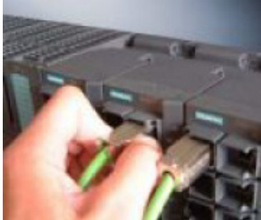
Figure 5-4 Releasing the RJ-45 Plug
