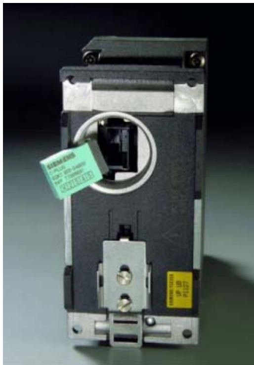
Figure 4-44 Removing the C-PLUG from the receptacle
