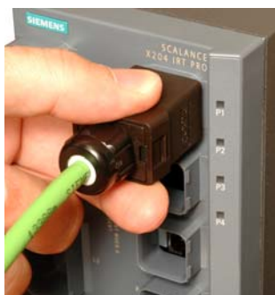
Figure 6-8 Removing IE RJ 45 Plug Pro or IE SC RJ Plug Pro
