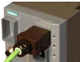
Figure 6-7 IE RJ 45 Plug Pro or IE SC RJ Plug Pro inserted
