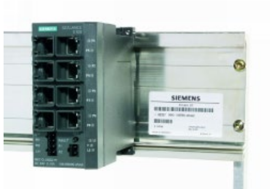
Image 4-3 Installation on a SIMATIC S7-300 standard rail
