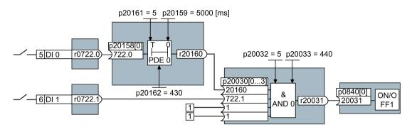
Figure A-7 Example: Signal interconnection for control logic
