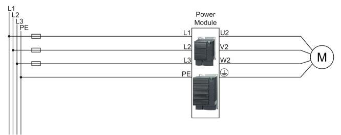
Figure 4-15 Connecting the PM260 Power Module
