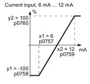
Set the following parameters to set the analog input as current input with monitoring:
