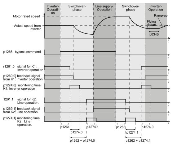
Figure 6-48 Bypass control independent of the speed via a control signal (p1267.0 = 1)
