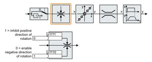
If you want to permanently enable the negative direction of rotation, then set parameter p1110 to 0.
