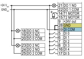
You must remove the jumper between terminals 28 and 69 if it is necessary to have electrical isolation between the external power supply and the internal inverter power supply.
