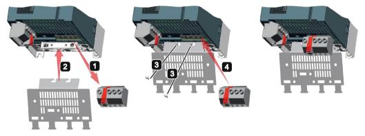
Figure 4-1 Mounting the shield plate, FSA ... FSC
