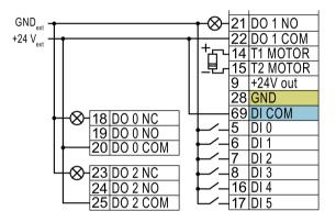
Remove the jumper between terminals 28 and 69.
