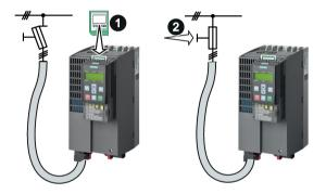
After the power supply has been switched on, the inverter copies its changed settings to the memory card.
