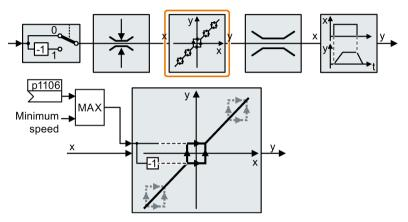
Speeds where the absolute value is less than the minimum speed are only possible during motor operation when accelerating or braking.
