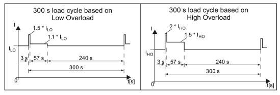
Figure 10-3 "Low Overload" and "High Overload" load cycles
