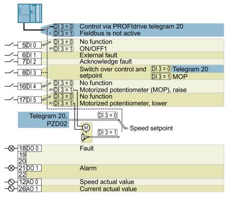
DO 0: p0730, DO 1: p0731 AO 0: p0771[0], AO 1: p0771[1] DI 0: r0722.0, ..., DI 5: r0722.5 Motorized potentiometer, setpoint after the ramp-function generator: r1050 Speed setpoint (main setpoint): p1070[0] = 2050[1], p1070[1] = 1050 Designation in BOP-2: Proc Fb
