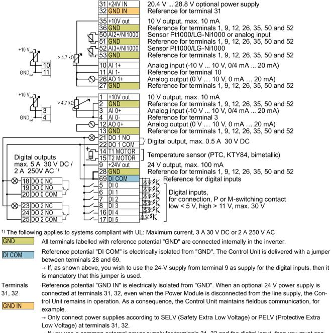
→ If you use a common external power supply for terminals 31, 32 and the digital input, then you must connect "GND" and "GND IN" with one another.
