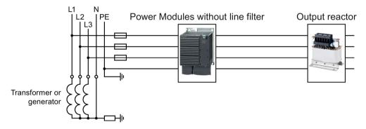
Figure 4-10 IT line supply where the neutral conductor N is transferred and with impedance with respect to the PE protective conductor
