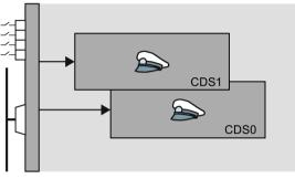
You select the command data set using parameter p0810. To do this, you must interconnect parameter p0810 with a control command of your choice, e.g. a digital input.
