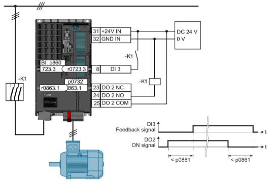
Figure 6-41 Line contactor control with monitoring
