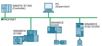
In PROFINET IO operation, the inverter supports the following functions:
