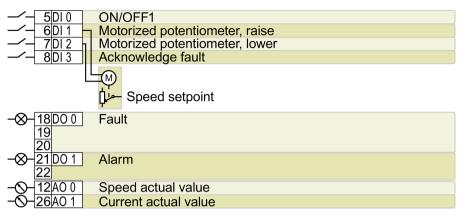
DO 0: p0730, DO 1: p0731 AO 0: p0771[0], AO 1: p0771[1] DI 0: r0722.0, ..., DI 3: r0722.3 Motorized potentiometer, setpoint after the ramp-function generator: r1050 Speed setpoint (main setpoint): p1070[0] = 1050 Designation in BOP-2: Std MoP
