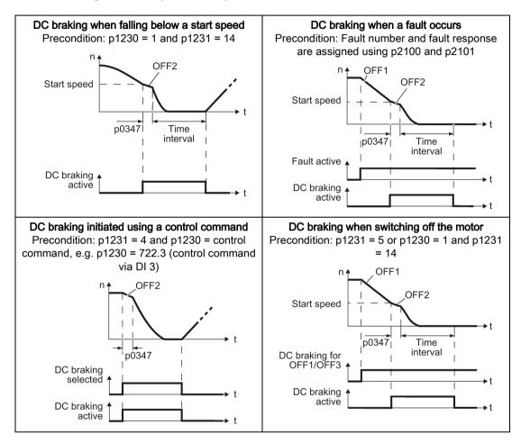
The DC-braking function is possible only for induction motors.
