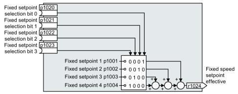
Figure 6-26 Simplified function diagram for directly selecting fixed setpoints
