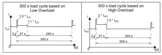
Figure 10-6 Load cycles "Low Overload" and "High Overload"
