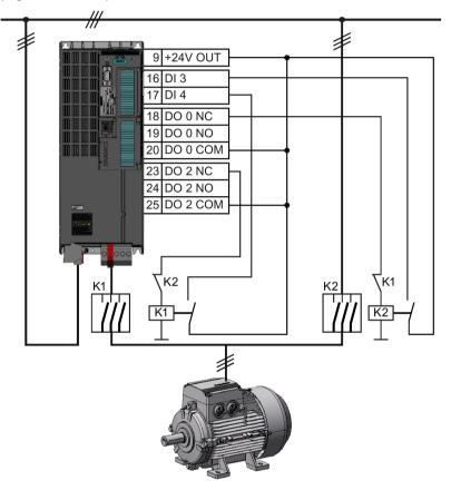
Figure 6-47 Bypass circuit for control using the inverter
