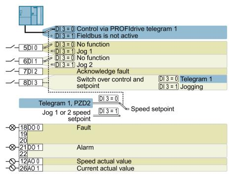
DO 0: p0730, DO 1: p0731 AO 0: p0771[0], AO 1: p0771[1] DI 0: r0722.0, ..., DI 3: r0722.3 Speed setpoint (main setpoint): p1070[0] = 2050[1] Jog 1 speed setpoint: p1058, factory setting: 150 rpm Jog 2 speed setpoint: p1059, factory setting: -150 rpm Designation in BOP-2: FB cdS
