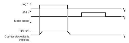
Figure 5-2 Jogging the motor in the factory setting
