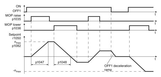
Figure 6-24 Function chart of the motorized potentiometer
