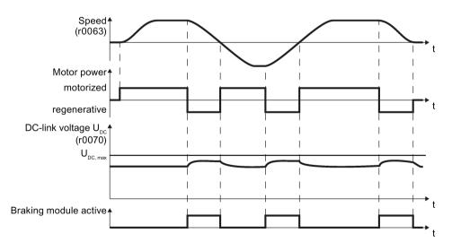
Figure 6-36 Simplified representation of dynamic braking with respect to time
