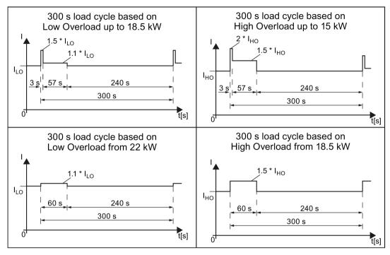
Figure 10-2 Duty cycles, "High Overload" and "Low Overload"
