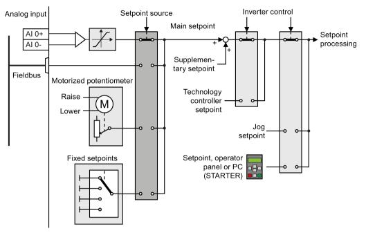
Figure 6-20 Setpoint sources for the inverter
