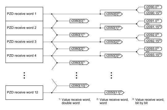
Figure 6-14 Interconnection of the receive words
