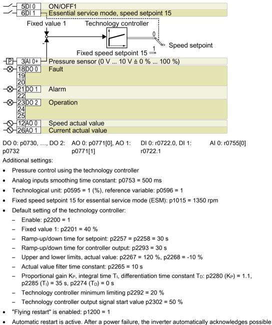
Automatic restart is active. After a power failure, the inverter automatically acknowle faults and switches on the motor: p1210 = 26
