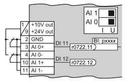
To use an analog input as additional digital input, you must interconnect the corresponding status parameter r0722.11 or r0722.12 with a binector input of your choice.
