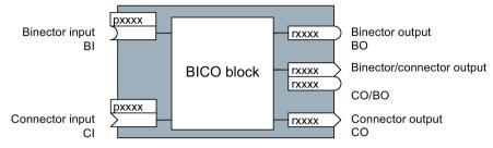
Figure A-6 Symbols for binector and connector inputs and outputs
