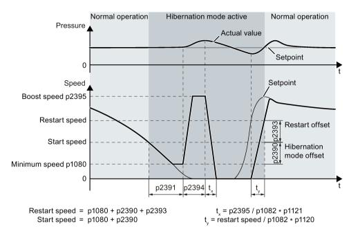
Figure 6-52 Hibernation mode using an external setpoint with boost
