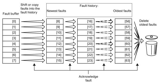
Figure 9-8 Fault history after acknowledging the faults
