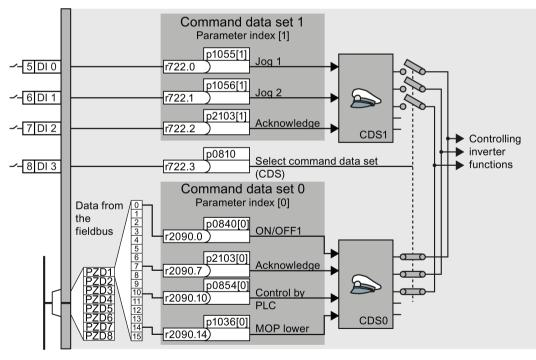
Figure 6-18 Example: Switching over the control via terminal strip to control via PROFIBUS or PROFINET
