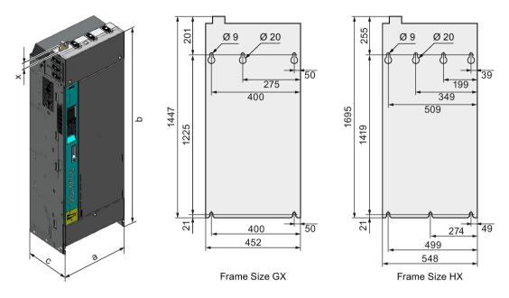
Dimensions and drilling patterns for the PM330 Power Modules:
