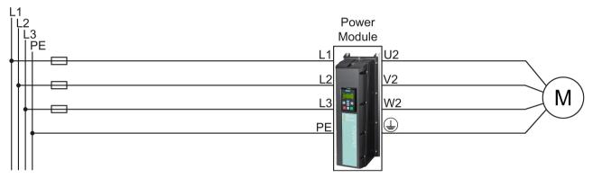
Figure 4-12 Connecting the PM230 IP55 Power Module
