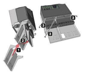
Figure 4-2 Mounting the shield plate, FSD ... PSF
