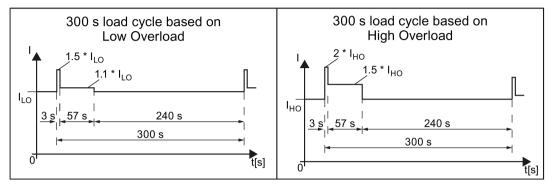
Figure 10-5 Load cycles "Low Overload" and "High Overload"
