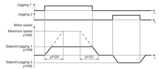
Figure 6-11 Behavior of the motor when "jogging"
