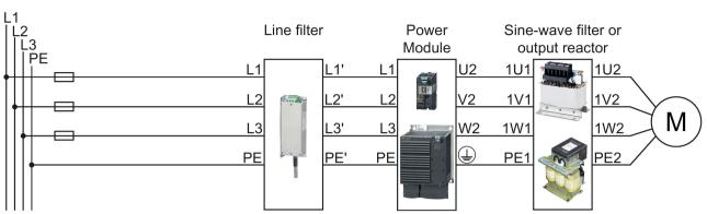
PM240 and PM240-2 Power Modules are available with and without integrated Class A line filters. For higher EMC requirements you need an external Class B line filter.
