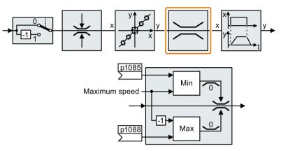
The converter generates a message (fault or alarm) when the maximum speed is exceeded.
