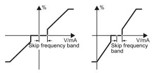
Interferences in the cable can corrupt small signals of a few millivolts. To be able to enter a setpoint of exactly 0 V via an analog input, you must specify a skip frequency band.
