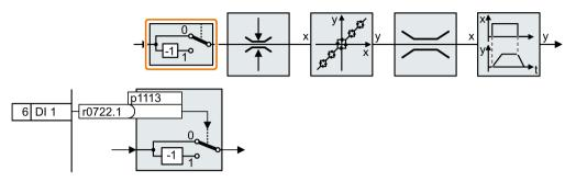
In order to invert the setpoint through the digital input DI 1, connect the parameter p1113 with a binary signal, e.g. the digital input 1.
