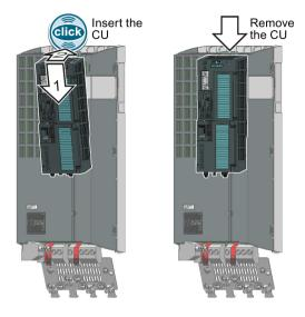
You have now plugged the Control Unit onto the Power Module.
