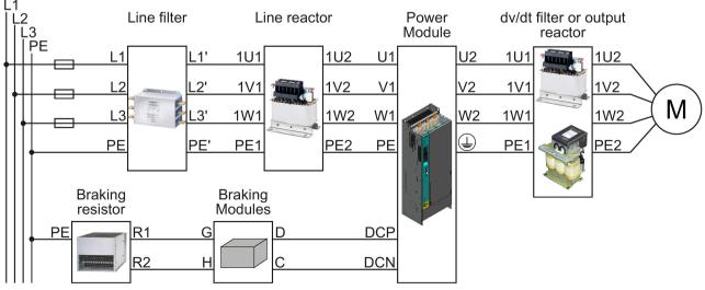
Figure 4-16 Connecting the PM330 Power Module
