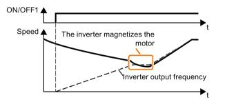
Figure 6-37 Principle of operation of the "flying restart" function
