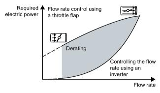
The converter calculates the energy saving from the flow characteristic associated with a mechanical flow control and the measured electric power that is drawn.
