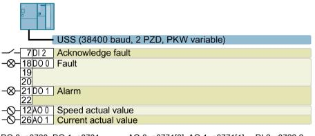
DO 0: p0730, DO 1: p0731 AO 0: p0771[0], AO 1: p0771[1] DI 2: r0722.2 Speed setpoint (main setpoint): p1070[0] = 2050[1] Designation in BOP-2: FB USS
