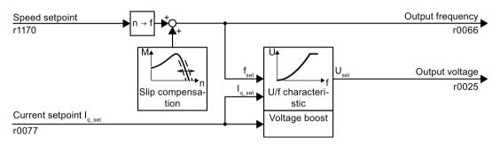
Figure 6-30 Default setting of the U/f control after selecting Standard Drive Control
