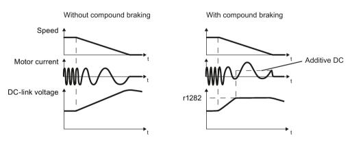
Figure 6-35 Motor brakes with and without active compound braking
