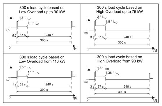
Figure 10-4 "High Overload" and "Low Overload" load cycles
