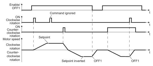
Figure 6-9 Three-wire control, method 1
