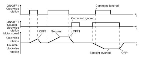
Figure 6-7 Two-wire control, method 2
