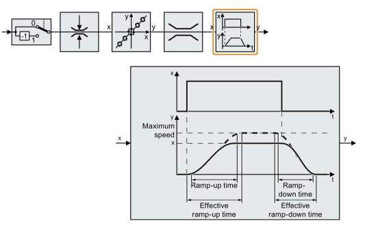
Initial and final rounding permit smooth, jerk-free acceleration and braking.
