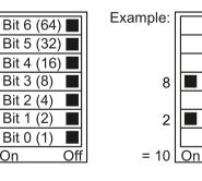
You set the PROFIBUS address of the inverter using the address switch on the Control Unit, in parameter p0918 or in STARTER.
