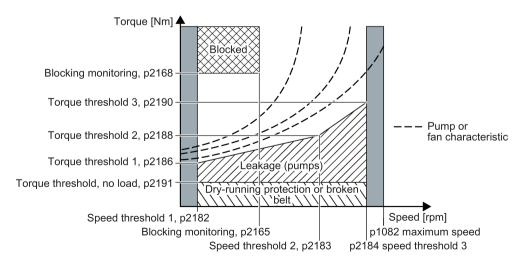
If the torque or the speed moves, for longer than the time set in p2192, in the ranges of blockage, leakage or dry running protection/belt breakage, then the response defined in p2181 is realized.
