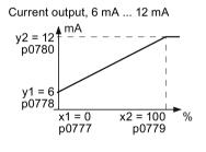
Set the following parameters to set the characteristic to match the example:
