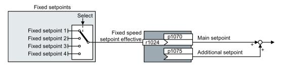
Figure 6-25 Fixed speeds as setpoint source
