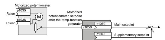
Figure 6-23 Motorized potentiometer as setpoint source
