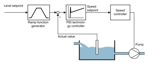
Figure 6-42 Example: Technology controller as a level controller
