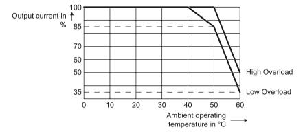
Current de-rating depending on the ambient operating temperature
