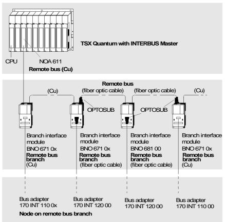
The conversion from copper cable to fiber optic cable is done with OPTOSUB or OPTOSUB PLUS, depending on the module used (see section *Transition from copper cable*  $\leftrightarrow$  *fiber optic cable*, *p. 12*).
