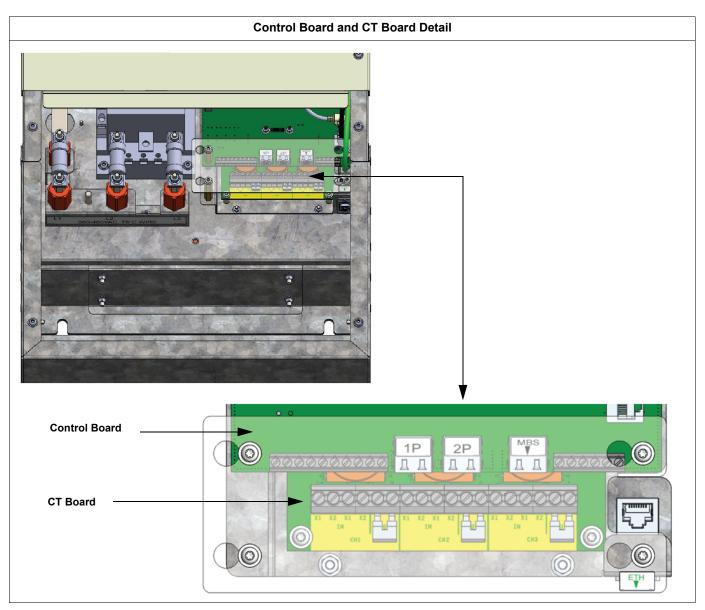
The terminal block on the CT board can accept wire sizes of up to 2.5  $\text{mm}^2$  (12 AWG) wire and has a torque specification of 1 N•m (9 lb-in).
