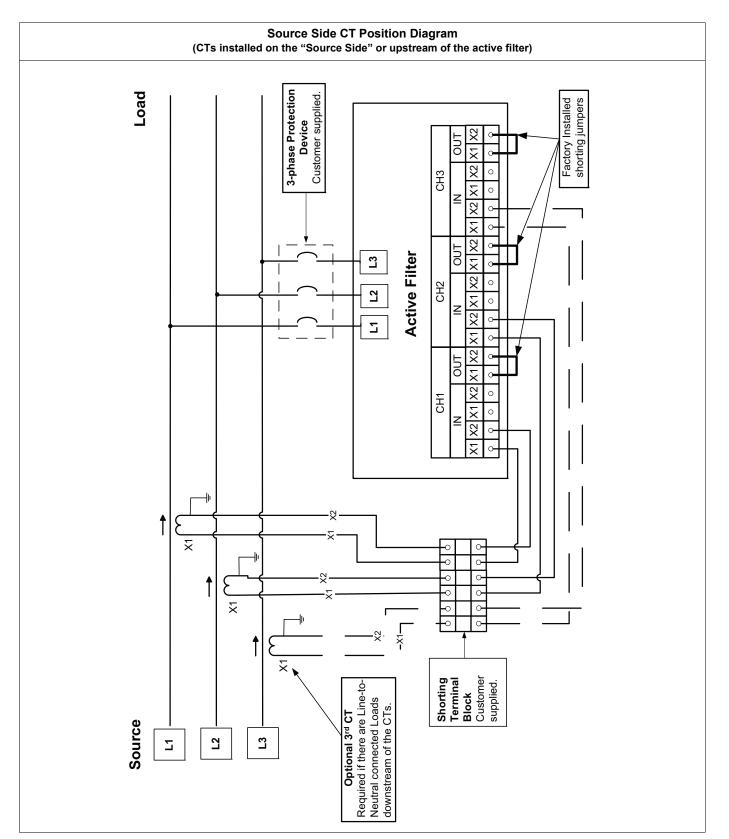
**NOTE:** The factory installed shorting jumpers must be installed.
