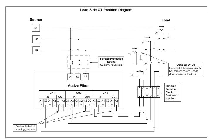
NOTE: The factory installed shorting jumpers must be installed.
