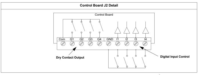
**NOTE:** The control board J2 accepts wire size between 0.2  $\rm{mm}^2$  (24 AWG) and 2.5  $\rm{mm}^2$  (12 AWG).
