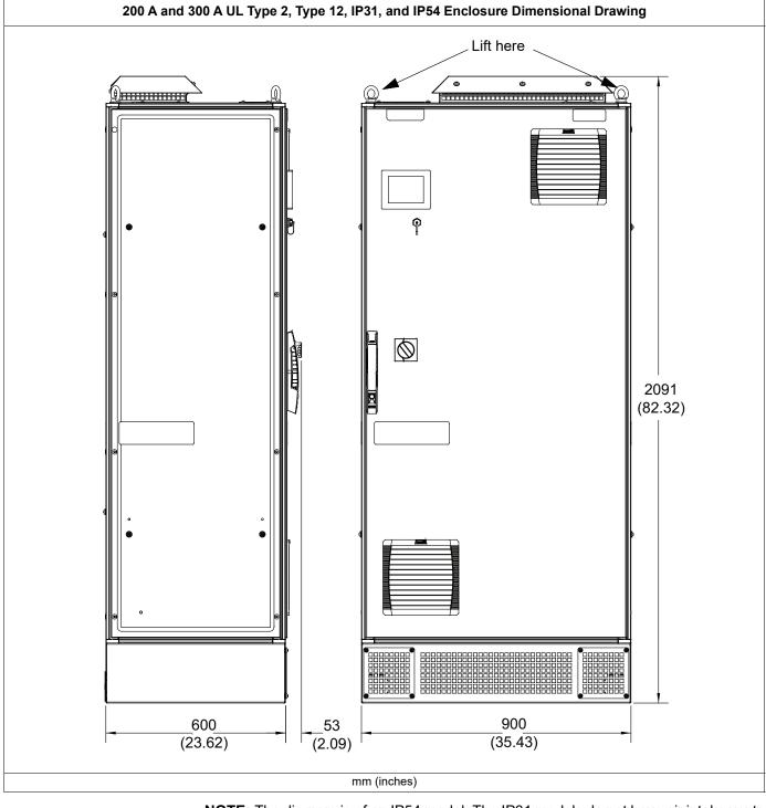
**NOTE:** The diagram is of an IP54 model. The IP31 models do not have air intake vents on the door.
