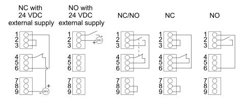
The EPO input supports 24 VDC.
