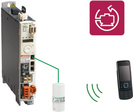
Configuration with SoMove Mobile software for cell phones via Bluetooth®
