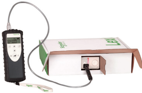
Configuration of a Lexium 32 in its packaging with the VW3A8121 Multi-Loader tool + VW3A8126 cordset
