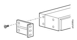
Install the PDU using the screws and caged nuts included with your rack or enclosure. The PDU will occupy 1 U-space.
