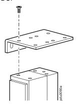
2. Install the PDU on a vertical mounting rail in your rack or enclosure.
